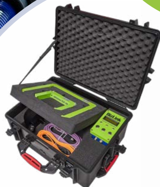
Mobile calibration case for the initial calibration of unknown tools and fixtures (TCP & Base)
